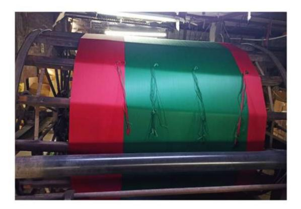
Powerloom warping is a process used to prepare yarn for weaving. It involves winding the yarn onto a beam in a specific pattern to create a warp. The warp is then used to create the fabric on a power loom. The process of powerloom warping is a complex one and requires a great deal of skill and experience.
