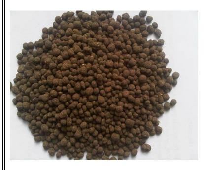
Press mud, the solid waste produced while processing sugar cane is rich in potassium, calcium, phosphorous and organic matters. Press mud is also a base material for producing bio-earth which is done by composting with spent wash, a liquid- waste generated out of distillery operation.
